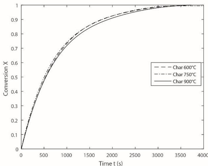
**Figure 5:** Influence of pyrolysis temperature on char conversion in an H<sub>2</sub>O atmosphere (partial pressure: 0.2 atm, temperature: 900°C)
