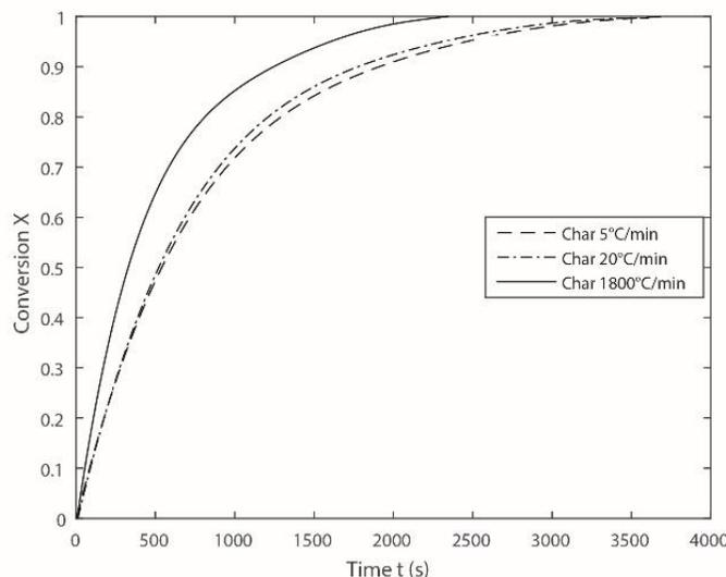
**Figure 6:** Influence of pyrolysis heating rate on char conversion in an H<sub>2</sub>O atmosphere (partial pressure: 0.2 atm, temperature: 900°C)
