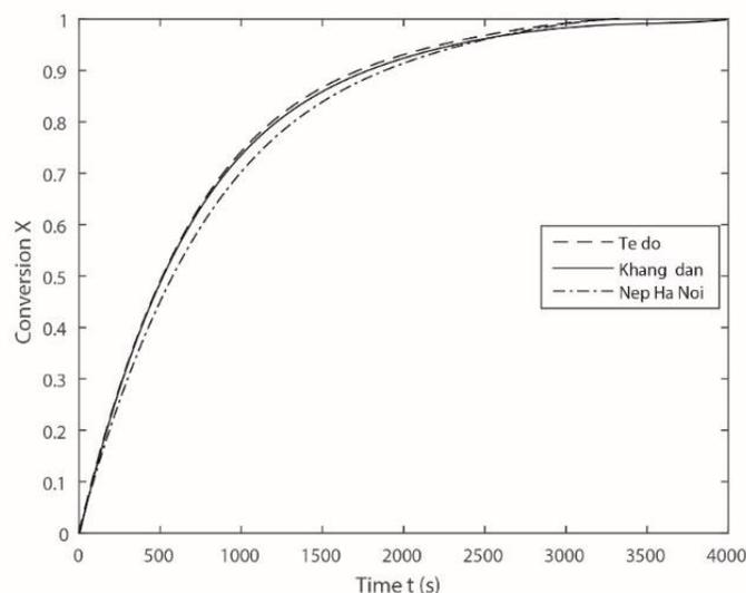
**Figure 7:** Influence of the nature of rice husk on char conversion in an  $\text{H}_2\text{O}$  atmosphere (partial pressure: 0.2 atm, temperature of reacting gas:  $900^\circ\text{C}$ ).
